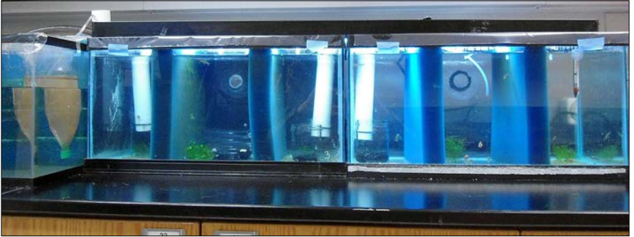
Figure 1: Three aquaria, with Poret foam subdivisions, connected by siphons. The white U-bend tubing links the three tanks. Water is pumped from one end to the other. The water is filtered of ammonia as it flows through the Poret foam from subdivision to subdivision. The setup takes up 1.2 m of bench-space.
