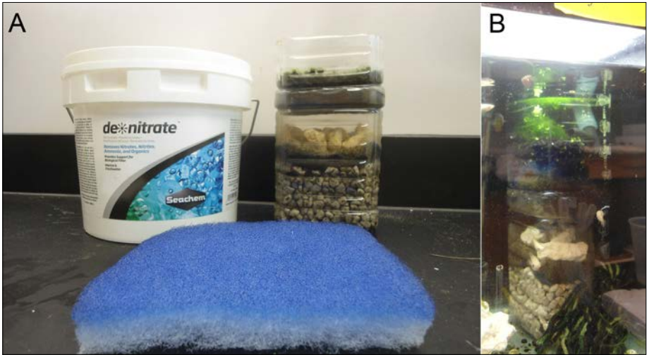
Figure 3: Home made canister filter. (A) The lower halves of juice bottles are stacked one on top of each other. The first layer is perforated and filled with activated carbon over some blue filter foam. The bottom layer is filled with Seachem De-Nitrate media with a layer of blue filter foam on top and a layer of crushed coral above that. (B) Water is pumped from one end of the series of aquaria and returned to the first compartment where it is directed into the filter. The carbon removes organic pollutants, the filter foam removes particulate matter, the crushed coral buffers the pH and the De-Nitrate media serves to both oxidize ammonia, reduce nitrate and manage nitrogen waste
